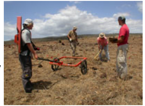
Using the GPS-enabled EM-61, a high-tech metal detector, workers conduct a subsurface search, mapping the location of anomalies beneath the surface.
